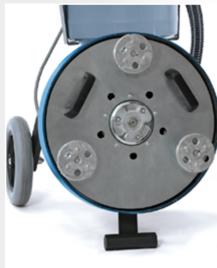
PLANETARY KS100 with 3 heads x 100 mm
