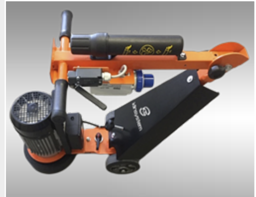
Folding handle for easy transport and facilitated storage
